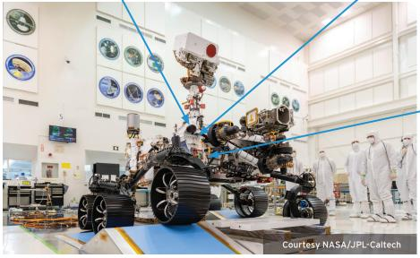
Sample handling assembly resolver Used to transfer the Mars surface core samples into a clean sample
