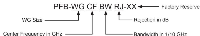
*Example: To order a WR-28 bandpass filter with 38 GHz center frequency, 2.2GHz bandwidth and 45 dB rejection, specify PFB-28382245-XX.*
